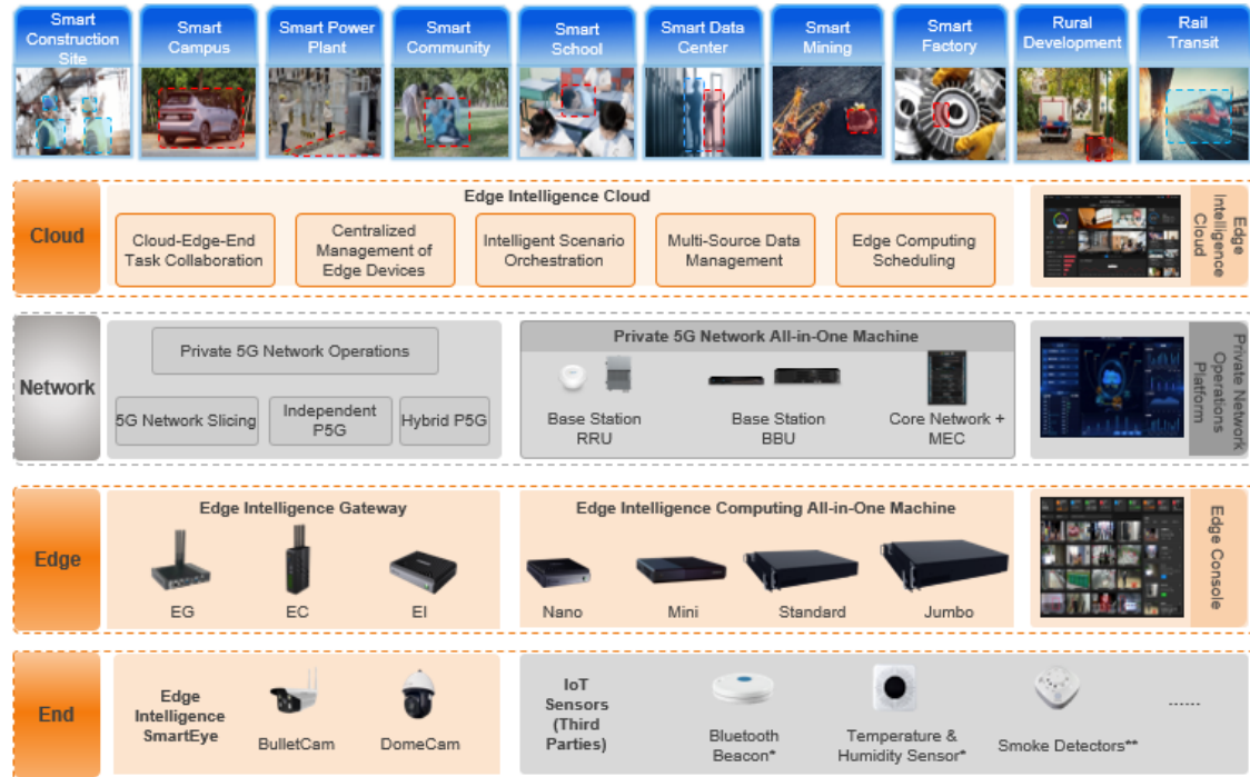
Figure 4-1 AISWare AI 2 Edge Intelligence Overall Architecture
